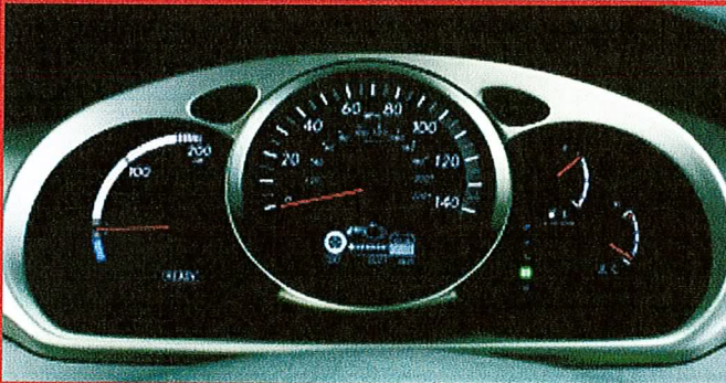
Technologically enhanced Optitron meter instrumentation with multi-information display and kW power meter.
