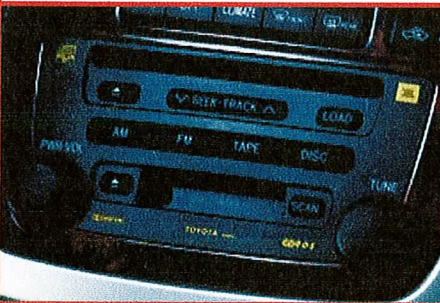
Available JBL 3-in-1 AM/FM Cassette/6-disc in-dash CD changer with eight speakers in six locations. 2
